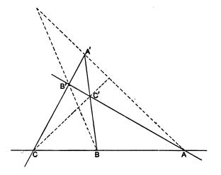
Let A, A'; B, B'; C, C'; be the three pairs of opposite vertices of the tetragram. Then evidently A and A' are a pair of centres of the tetrastigm BC, B'C'. Hence, by § 141, it follows that BB', and CC', cut AA' in two points which are harmonic conjugates with respect to A and A'.
